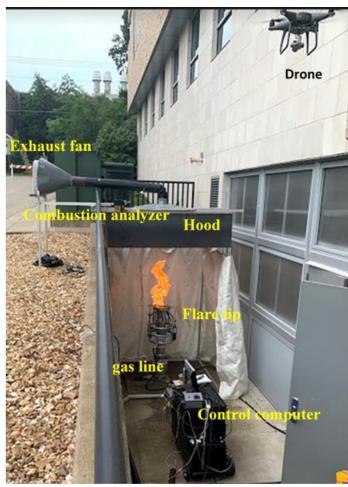
Figure 2 - Flare Test Setup
