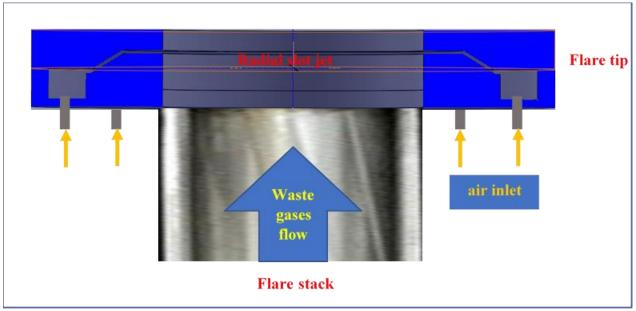
Figure 1 – Aero-nozzle flare tip design
