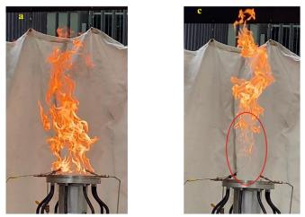
Figure 5 - Flame above Flare Tip with 20 L/min propane with: a) 0 cfm assist air, b) 10 cfm assist air
