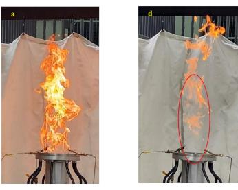
Figure 6 - Flame above Flare Tip with 20 L/min propane with: a) 0 cfm assist air, b) 12 cfm assist air
