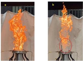
Figure 4 - Flame above Flare Tip with 20 L/min propane with: a) 0 cfm assist air, b) 8 cfm assist air
